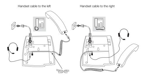
You can put the cable to the handset in the notch underneath the telephone. The cable to the exchange has to be plugged in LINE and the handset cable has to be plugged in HANDSET.
